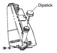
8. Remove the dipstick and check the oil level. Add oil as needed. Maintain the oil level in the safe range. Do not overfill.
